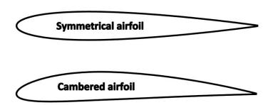
The difference between a cambered airfoil such as found on a transport category aircraft and a symmetrical airfoil common to modern high performance light aerobatic aircraft.
